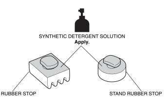
2. Install the rubber stop in the positions shown.
