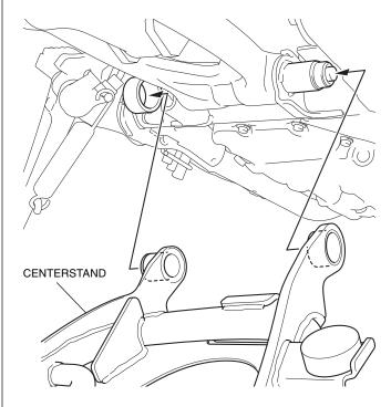
Install the circlip and washer as shown.
