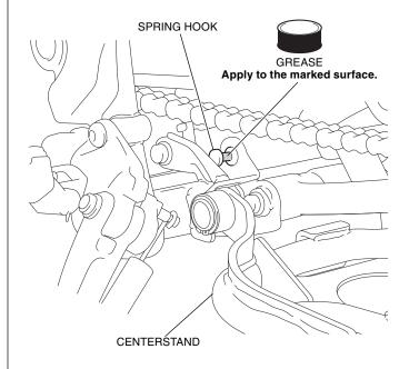
10. Install the spring plate as shown.
